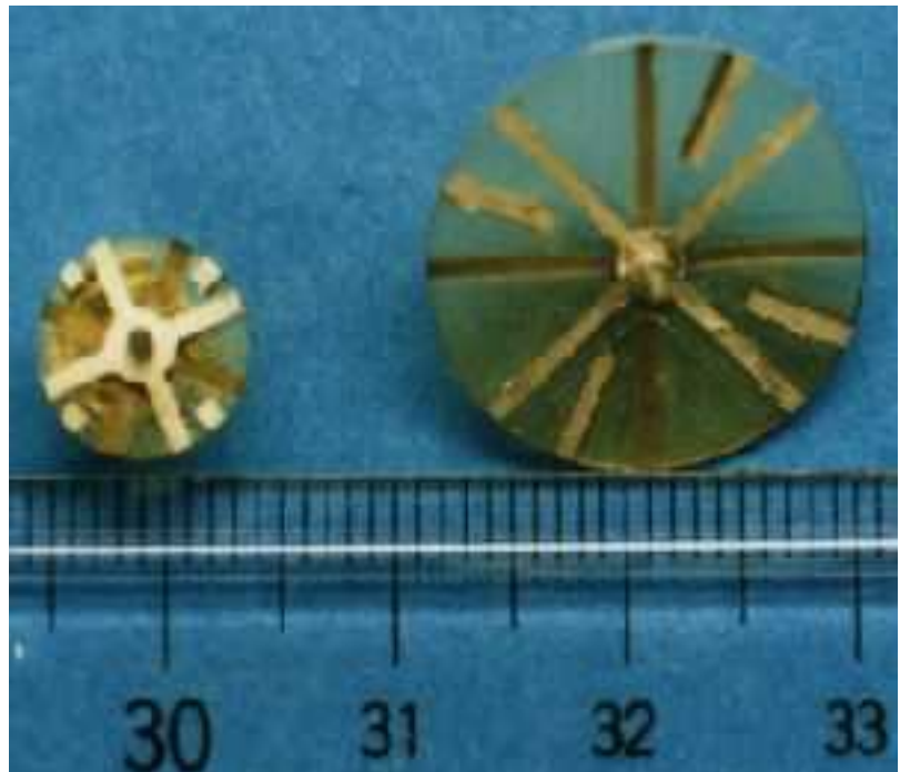
Fig.10-2 Rotor of DP-RE type ECF Motor
