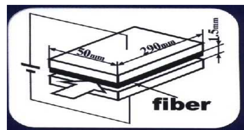
Fig.11 -2: ECF Valve system
