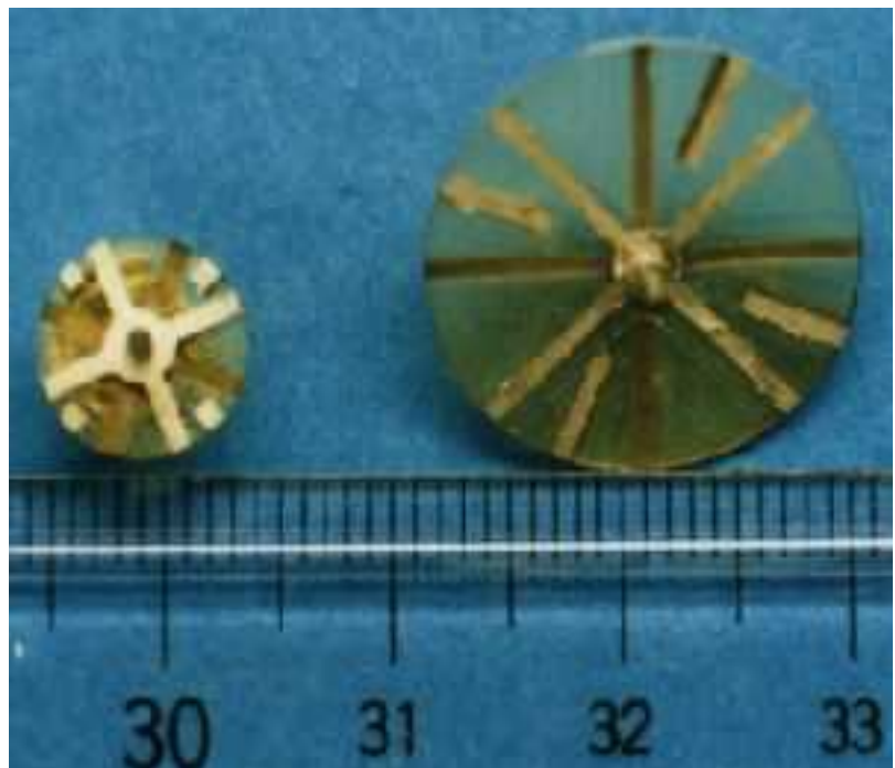
Fig.10-2 Rotor of DP-RE type ECF Motor
