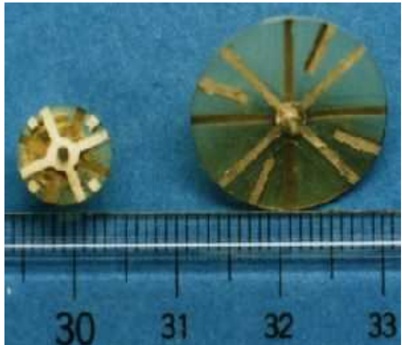
Fig.10-2 Rotor of DP-RE type ECF Motor
